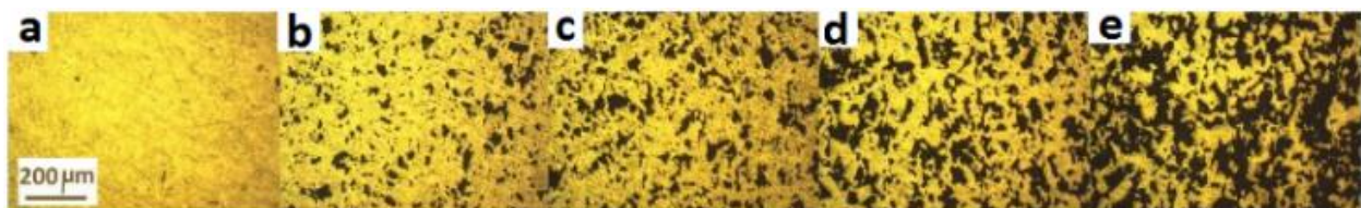
Figure 5. Different layers of the FGM sample; a) Ti, b) Ti/10 vol% HA, c) Ti/20 vol% HA, d) Ti/30 vol% HA and e) Ti/40 vol% HA.
