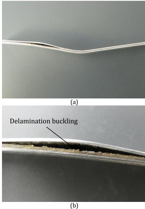
Figure 8. (a) Photographs of failure modes following flexural testing in the FML/TF specimens, (b) magnified at fracture surface
