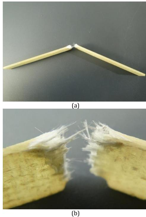
Figure 10. (a) Failure modes following impact testing in the GE/TF specimens, (b) magnified at fracture surface
