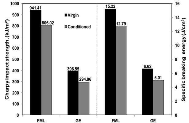
Figure 9. Charpy impact strength and specific breaking energy of the FMLs and GE composites before and isothermal aging
