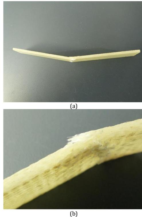
**Figure 7.** (a) Photographs of failure modes following flexural testing in the GE/TF specimens, (b) magnified at fracture surface
