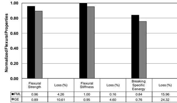
Figure 6. Degradation of flexural properties of FML and GE laminates after exposure to the isothermal aging
