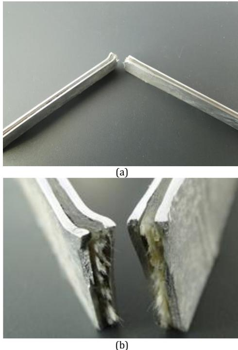
**Figure 11.** (a) Failure modes following impact testing in the FML/TI specimens, (b) magnified at fracture surface
