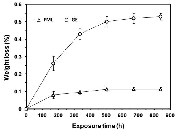
Figure 3. Percentage weight loss of GE and FML specimens subjected to isothermal aging at  $130^\circ\text{C}$
