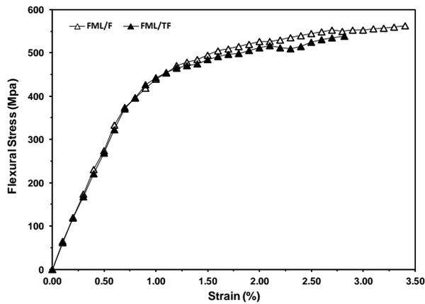
Figure 4. Typical flexural stress-strain curves for FML laminates before and after exposure to isothermal aging
