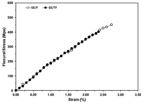
Figure 5. Typical flexural stress-strain curves for GE laminates before and after exposure to isothermal aging
