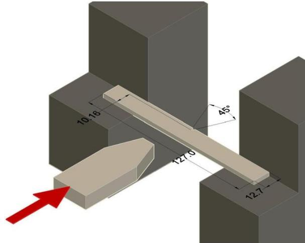
Figure 2. Schematic Charpy test specimen prepared according to ASTM D 6110 (All dimensions are in mm)
