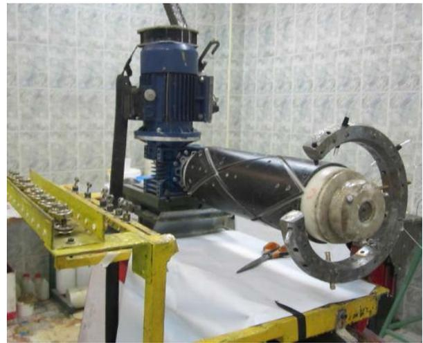
Figure 1. Filament winding apparatus
