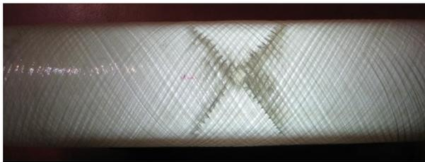
**Figure 6.** Tube with 0.5 wt% nanoparticles
