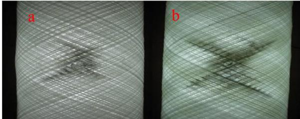
**Figure 4.** a) Sample with 0wt% nanoparticles; b) Sample with 3wt% nanoparticles.
