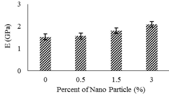
Figure 3. Elastic modulus by weight percentage of silica nanoparticles
