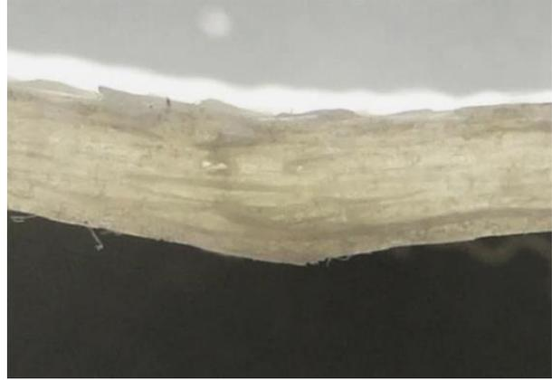
Figure 6. Photographs of failure modes following flexural testing in the GE/Dry specimens
