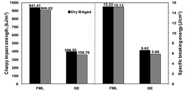
Figure 14. Charpy impact strength and specific breaking energy of the FMLs and GE composites before and after hygrothermal aging
