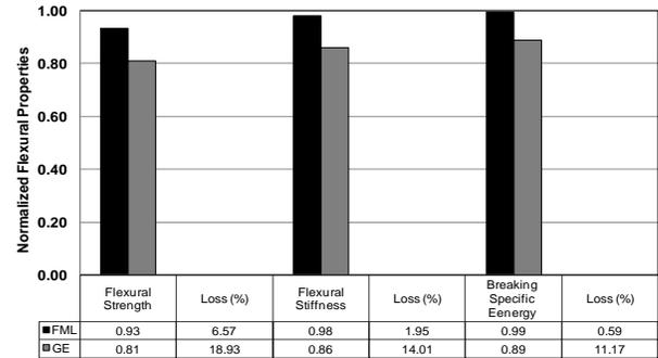
**Figure 5.** Degradation of flexural properties of FML and GE laminates after exposure to the hygrothermal aging
