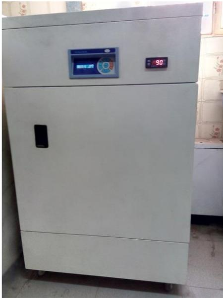
Figure 1. Hygrothermal test chamber
