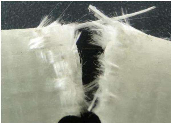
**Figure 11.** Photographs of failure modes following impact testing in the GE/Dry specimens
