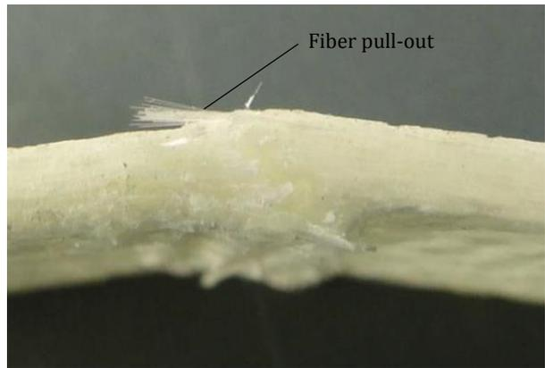
Figure 7. Photographs of failure modes following flexural testing in the GE/Aged specimens
