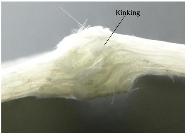
**Figure 12.** Photographs of failure modes following impact testing in the GE/Aged specimens
