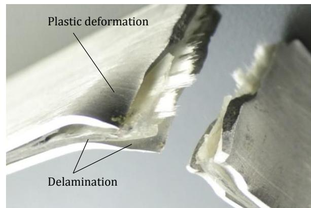
**Figure 14.** Photographs of failure modes following impact testing in the FML/Aged specimens
