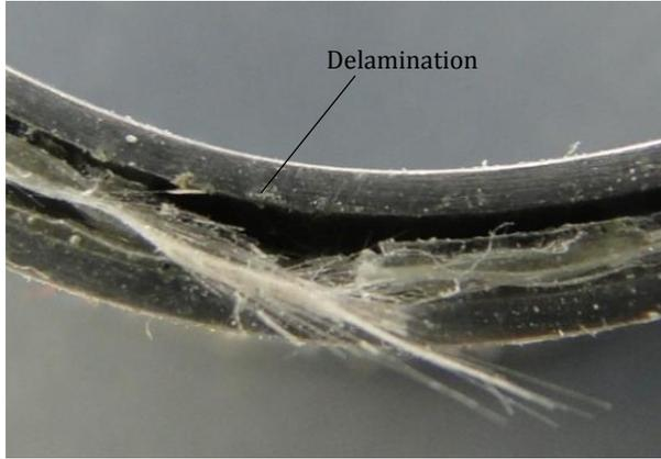
Figure 9. Photographs of failure modes following flexural testing in the FML/Aged specimens
