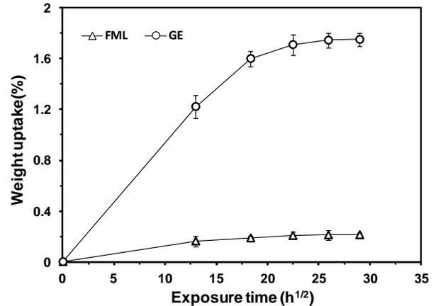
Figure 2. Water absorption curves of FML and GE laminates immersed in water at  $90 \text{ }^\circ\text{C}$
