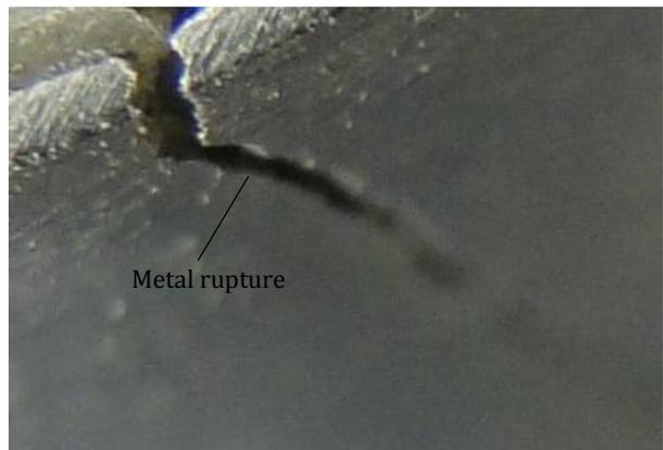
Figure 8. Photographs of failure modes following flexural testing in the FML/Dry specimens
