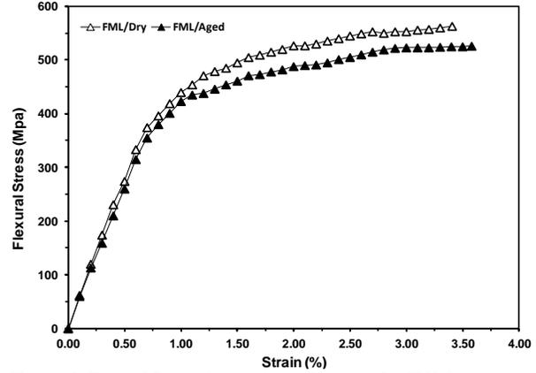
**Figure 3.** Typical flexural stress-strain curves for FML laminates before and after exposure to hygrothermal aging
