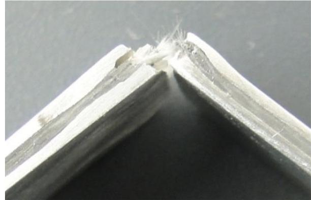
**Figure 13.** Photographs of failure modes following impact testing in the FML/Dry specimens
