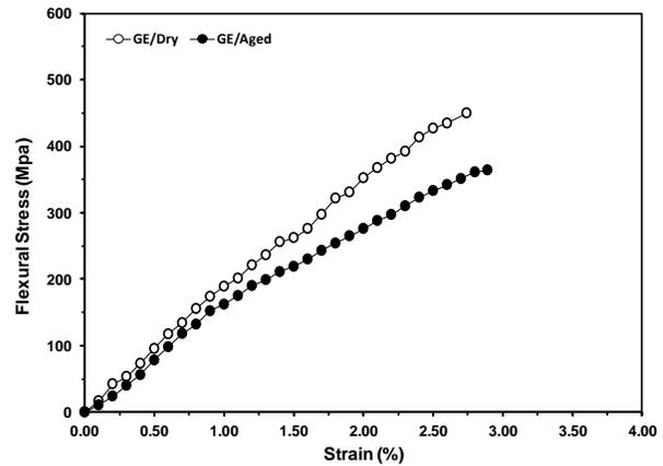
**Figure 4.** Typical flexural stress-strain curves for GE laminates before and after exposure to hygrothermal aging
