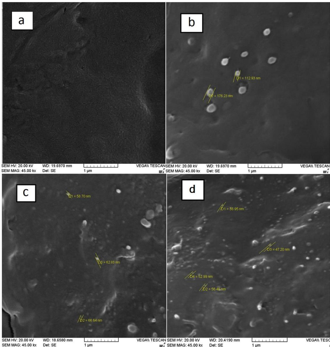
**Figure 6.** SEM micrographs of (a) neat PP, (b) PP/MCM-41-HA nanocomposite (temperature 170° C and rotational speed of 50 rpm), (c) PP/MCM-41-HA nanocomposite (temperature 180° C and rotational speed of 50 rpm), (d) PP/MCM-41-HA nanocomposite (temperature 180° C and rotational speed of 100 rpm).
