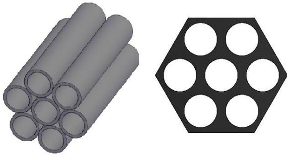
**Figure 1.** The schematic form of mesoporous silica nanoparticles.
