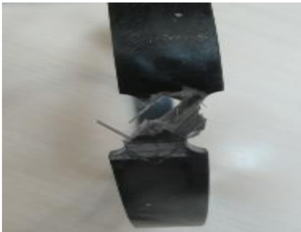
Figure 13. The hoop specimen after the complete fracture
