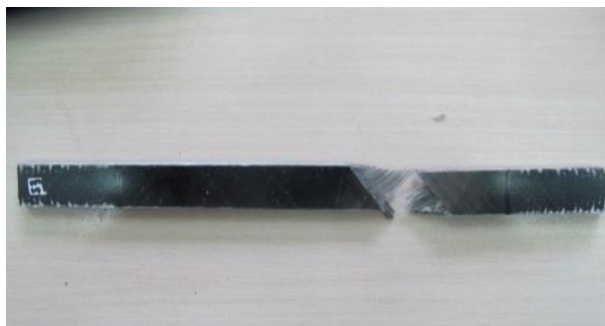
Figure 8. The longitudinal specimen after a complete fracture
