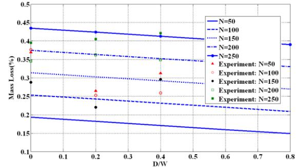
Figure 6. Mass loss of unnotched and open-hole  $[0_2/90_2]_s$  specimens due to oxidation
