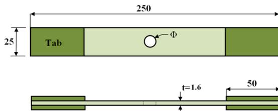
**Figure 1.** Test specimens with open hole
