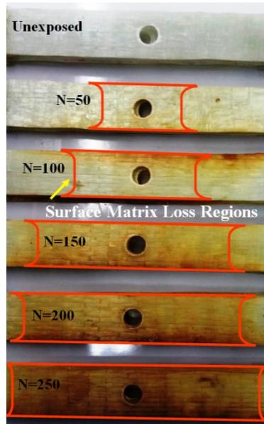
Figure 3. Growth of the surface-degradation regions during thermal cycle
