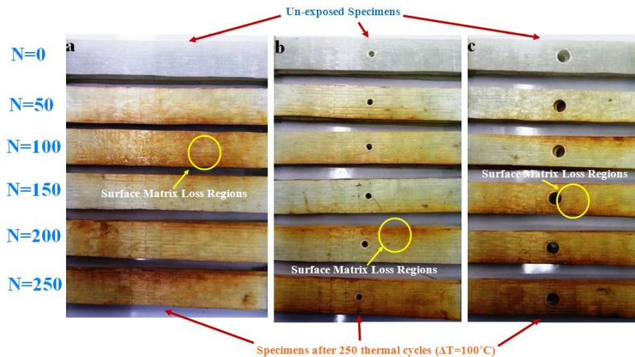
Figure 4. Surface degradation under the thermal cycling in a) unnotched, b) 5 mm open-hole, and c) 10 mm open-hole specimens.
