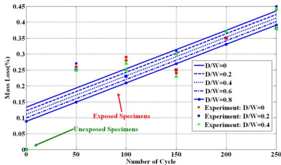
Figure 5. Variation of the mass loss as a function of the number of thermal cycles
