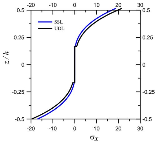
**Figure 6.** Through-thickness variations of  $\bar{\sigma}_x$  in  $0^\circ/90^\circ/0^\circ$  laminated beams subjected to single sinusoidal and uniformly distributed loading at  $L/h = 4$ .
