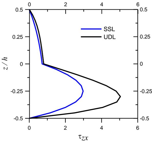
**Figure 4.** Through-thickness variations of  $\bar{\tau}_{zx}$  in  $0^\circ/90^\circ$  laminated beams subjected to single sinusoidal and uniformly distributed loading at  $L/h = 4$ .
