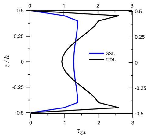
**Figure 10.** Through-thickness variations of  $\bar{\tau}_{zx}$  in sandwich beams subjected to single sinusoidal and uniformly distributed loading at  $L/h = 4$ .
