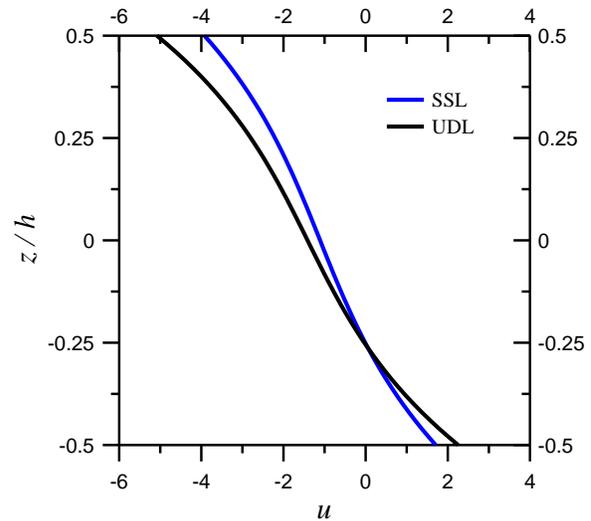
**Figure 2.** Through-thickness variations of  $\bar{u}$  in  $0^\circ/90^\circ$  laminated beams subjected to single sinusoidal and uniformly distributed loading at  $L/h = 4$ .
