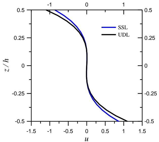
**Figure 5.** Through-thickness variations of  $\bar{u}$  in  $0^\circ/90^\circ/0^\circ$  laminated beams subjected to single sinusoidal and uniformly distributed loading at  $L/h = 4$ .
