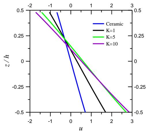
**Figure 11.** Through-thickness variations of  $\bar{u}$  in functionally graded beams subjected to single sinusoidal loading at  $L/h = 4$ .
