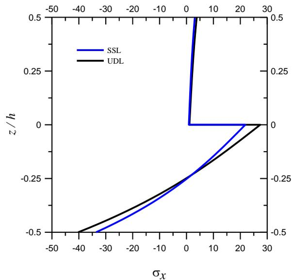
**Figure 3.** Through-thickness variations of  $\bar{\sigma}_x$  in  $0^\circ/90^\circ$  laminated beams subjected to single sinusoidal and uniformly distributed loading at  $L/h = 4$ .
