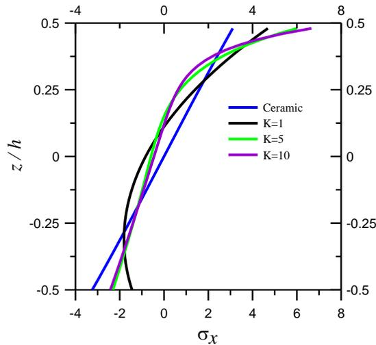
**Figure 12.** Through-thickness variations of  $\bar{\sigma}_x$  in functionally graded beams subjected to single sinusoidal loading at  $L/h = 4$ .
