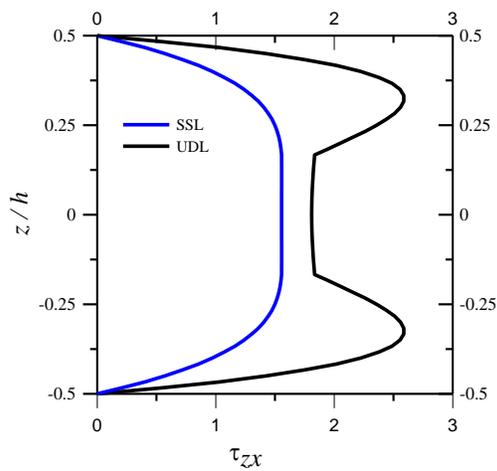
**Figure 7.** Through-thickness variations of  $\bar{\tau}_{zx}$  in  $0^\circ/90^\circ/0^\circ$  laminated beams subjected to single sinusoidal and uniformly distributed loading at  $L/h = 4$ .
