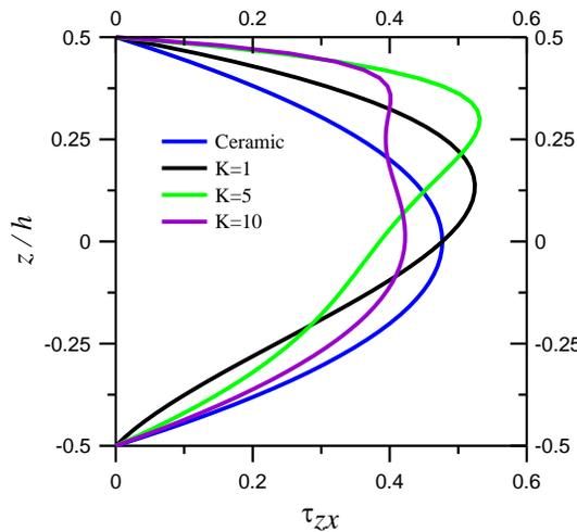
**Figure 13.** Through-thickness variations of  $\bar{\tau}_{zx}$  in functionally graded beams subjected to single sinusoidal loading at  $L/h = 4$ .
