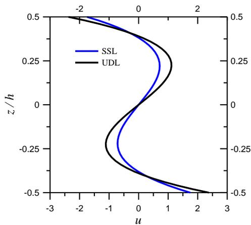
**Figure 8.** Through-thickness variations of  $\bar{u}$  in sandwich beams subjected to single sinusoidal and uniformly distributed loading at  $L/h = 4$ .
