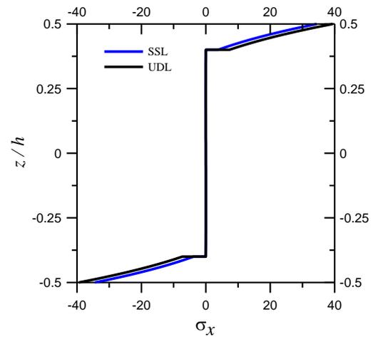
**Figure 9.** Through-thickness variations of  $\bar{\sigma}_x$  in sandwich beams subjected to single sinusoidal and uniformly distributed loading at  $L/h = 4$ .
